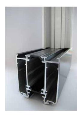
The ST Door offers high levels of both thermal insulation achieving a U value of 2.2 W/m2K. This low U value can help building designers to achieve their Target Emissions Rate (TER) by being offset against the allowable U value of 3.5 W/m2K for high traffic doors when calculating the Building Emissions Rate (BER).
