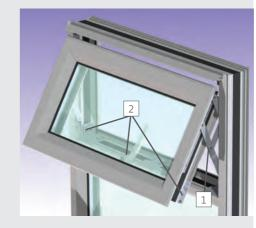
2. A turn of the handle operates the shootbolt locking mechanism and drives high strength brass alloy bolts into the window frame into die-cast keeps in the outer frame. The locking mechanism also offers a lockable 'night-vent' position.
