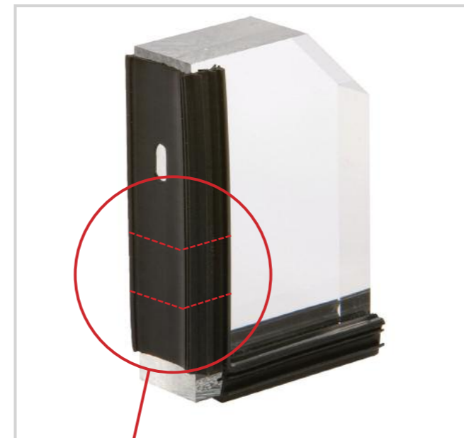
Wrap around glazing gasket perforated at 10mm intervals which breaks into harmless pieces when there is an attempt to remove it
